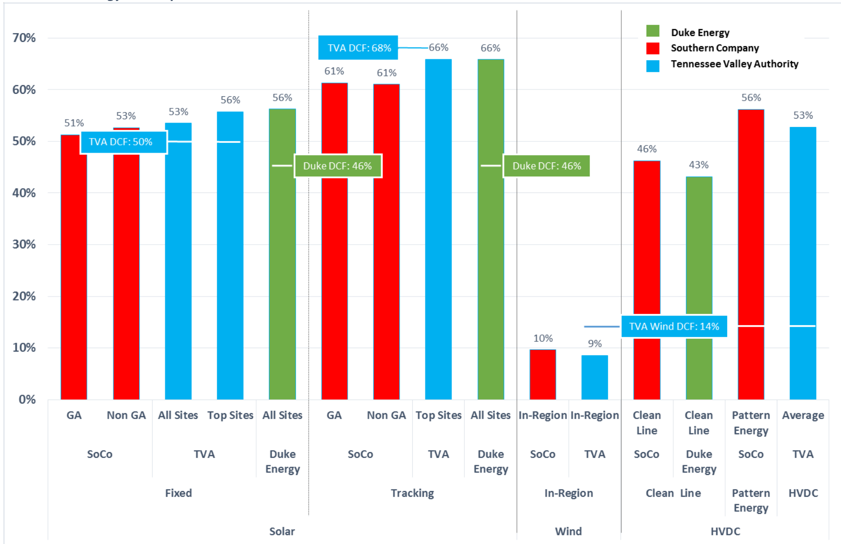
Figure 2: Summer Dependable Capacity Factors Calculated Using System Peak Hours Method, Assuming No Substantial Prior Renewable Energy Development
