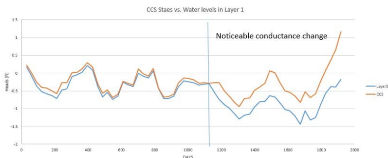
Figure 16. Simulated water levels in the CCS canal and model Layer 1 in monthly calibration model.
