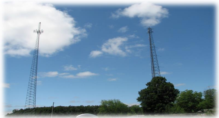
Two monitoring towers in Arkansas used to collect data on wind speeds. Credit: AWS Truepower, LLC
