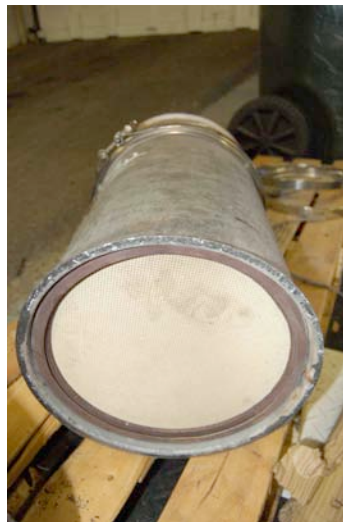
Figure 1: The honeycomb cross-section of a DPF. In theory, build-up of backpressure in the engine may result from the honeycomb design, resulting in loss of fuel efficiency and an increase in fuel use. Based upon the best available data, the calculations in this paper conservatively assume that a DPF retrofit on a large commercial truck may result in a 2 percent fuel penalty.
