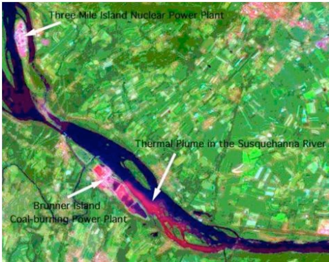
Figure 3. Landsat Image of Three Mile Island Nuclear and Brunner Island Coal Plants 5
