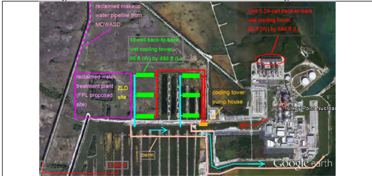
Figure 12. 54-Cell Back-to-Back Mechanical Draft Cooling Towers
