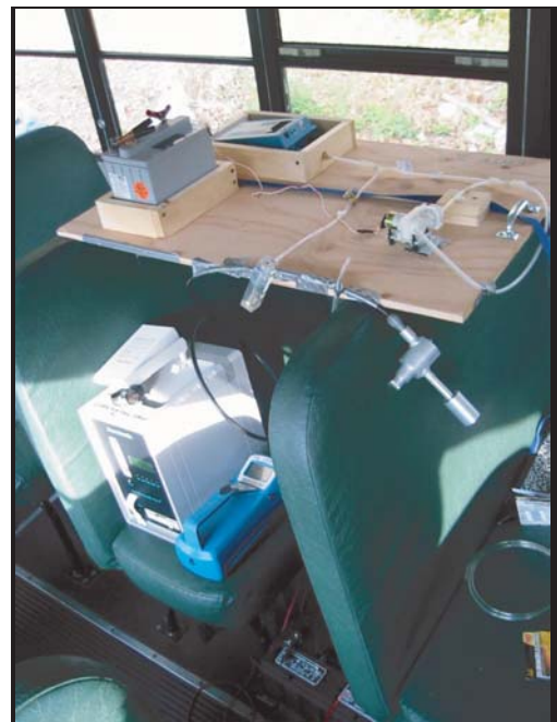
Testing Equipment: TSI/Dust trak, TSI/Ptrak monitor and Magee Scientific Aethalometer
