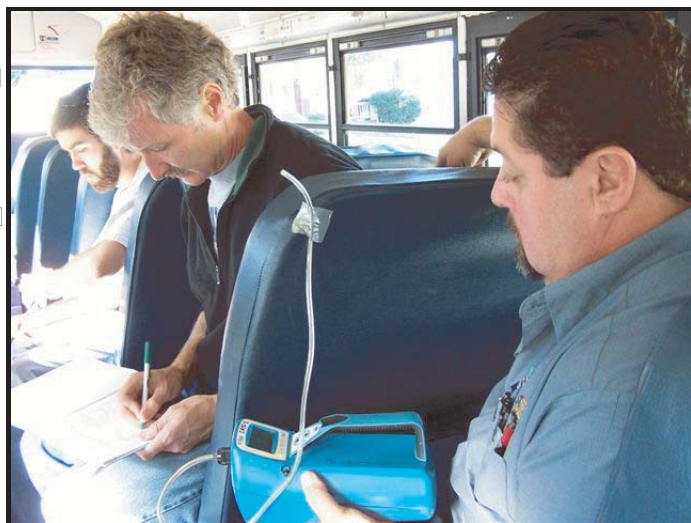
L. Bruce Hill, principal investigator, with volunteer. They are tracking measurements of ultrafine particles with a PTrak monitor.
