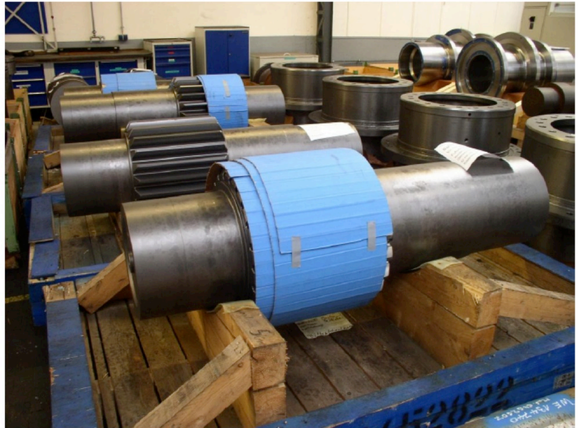
4 offset planet shaft after hardening
