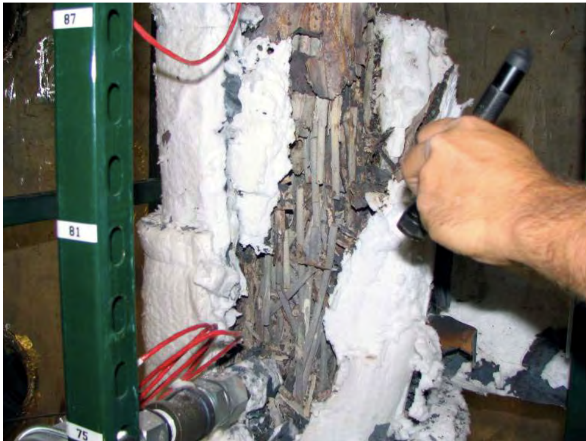
Figure VIII-2 Outcome of Test Burn of a BWR Fuel Assembly
